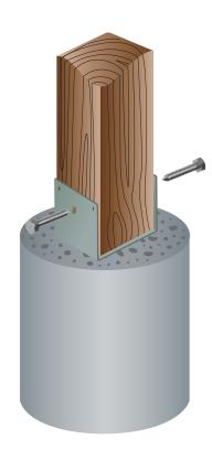
4. Insert post into post holder and attach with 2 lag screws.
