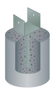
2. Insert post holder into concrete and level post holder.
