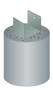
3. Smooth concrete around post holder. IMPORTANT: allow concrete to cure before installing post.
