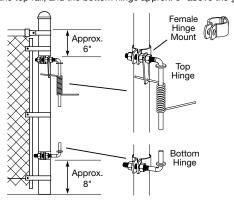
Secure hinge clamps to gate frame but do not fully tighten. The truss wire on the gate should be at the top corner of the hinge side of the gate. Adjust the position of the gate hinge clamps so that the top of the gate is level with the top rail of the fence. Tighten the hinge clamp bolts to secure the position of the gate.
