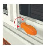
11. Position plastic handles on vertical frame at desired height. Drill 1/8" pilot holes and attach the handles with four flat head screws (provided).
