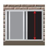
2. Square-cut vertical frames to measured height less 3-1/2".
