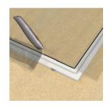
8. Insert rubber gasket down the side of the vertical frame. Use knife to trim excess length. Optional: If strip is too wide, cut off excess along grooved lines.
