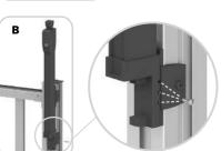
A: Adjust the vertical position of the latch until the marks line up on the latch and striker.
