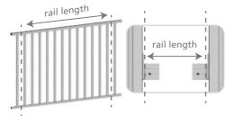
**If required,** cut the rails to fit between the brackets.
