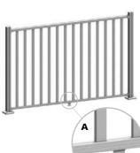
Fasten the second post to the concrete surface (see Step 1). Install bottom rail support:
