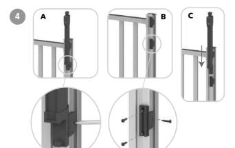
**A:** Position the latch at the required height on the fence post and then mark the location of both latch brackets (maximize distance between brackets).
