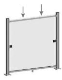
Install the top rail into the top brackets, ensuring the glass panel is fully engaged in the glass gasket.
