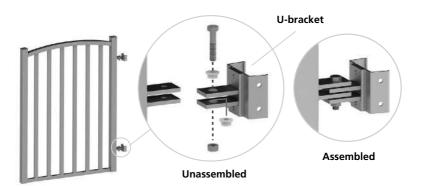
Install each hinge and U-bracket assembly on the gate and secure with bolt, bushings and nut (provided). For wooden posts only: Do not use the U-bracket.
