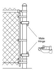
Attach gate to post by placing bottom gate frame hinge onto pin of bottom gate post hinge. Then, lower pin of top gate post hinge into gate frame hinge and tighten.
