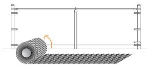
To remove excess fencing fabric, use pliers to open top & bottom 'knuckles' (where wires are locked together) and unweave one of the wires.
