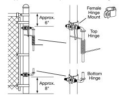
Secure hinge clamps to gate frame but do not fully tighten. The truss wire on the gate should be at the top corner of the hinge side. Adjust the position of the gate hinge clamps so that the top of the gate is level with the top rail of the fence. Tighten the bolts to secure the position of the gate.
