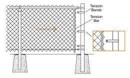
Install a temporary tension bar approx. 3 feet from final main post. Using a fence stretcher, stretch fence towards final main post and attach mesh to final main post with another tension bar and tension bands. Do not over-stretch the fence fabric - it should have a slight amount of movement when squeezed by hand. Once securely installed, release fence stretcher and remove temporary tension bar.
