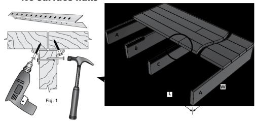
Installation Nail or screw hidden deck fasteners to the inside edges of outer joists (A), alternate edges of inner joists (B), and both edges of joists where decking is spliced (C), as shown above. Hammer nails in every other hole of the hidden deck fastener. Starting at one end of the joists, attach deck boards with two screws at each joist. (Fig. 1)
