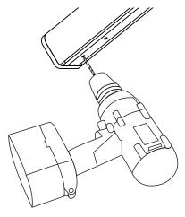
**15.** Secure end caps with a self-tapping screw (provided) at each end of handrail.
