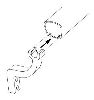
**10.** With the help of another person, adjust the handrail height and slide the brackets into the marked positions. Then follow step 3 to attach the brackets to the wall.
