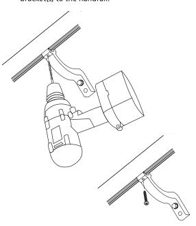
**12.** Drill <sup>3</sup>/<sub>16</sub>" pilot holes and fasten each bracket to the wall with a second lag screw (provided). Tighten the lag screws on all brackets.
