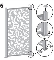
Fasten second post in place (see Step 1 for full details). Install post caps and post base covers.
