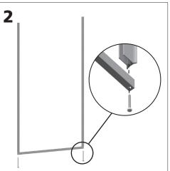
Secure Bottom Frame to two Vertical Frames using two #10 x 2" screws.
