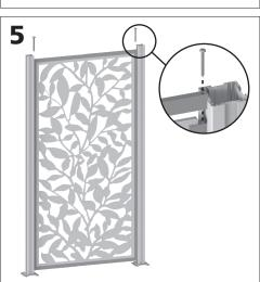
Position Top Frame onto 3' x 6' Decorative Screen and secure using two #10 x 2" screws.
