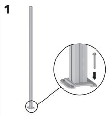
Position first post. For concrete attachment, use hammer drill with 5/16" masonry bit to drill four holes 3" deep through each corner of post base Clean holes. Use hammer to insert assembled concrete anchors (provided) until washer is touching post base. Use 7/16" wrench to tighten nuts. Ensure post is plumb.
