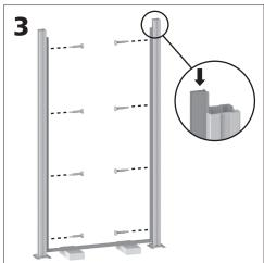
Position second post (do not secure it yet). Slide assembled Bottom Frame and Vertical Frames into assembled Bottom Frame and Vertical Frames into slots on posts and use wood blocks to level. Ensure bottom of frame is between 1-1/2" and 2" above ground. Secure Vertical Frames to posts using eight #10 x 1" self-drilling screws (provided).
