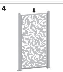
Slide 3' x 6' Decorative Screen down into Vertical Frames and ensure it is fully seated in Bottom
