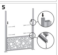
Secure one Mid Frame to two Vertical Frames using two #10 x 2" screws. Slide assembled Mid Frame and Vertical Frames into slots on posts.
