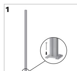
Position first post. For concrete attachment, use hammer drill with 5/16" masonry bit to drill four holes 3" deep through each corner of post base. Clean holes. Use hammer to insert assembled concrete anchors (provided) until washer is touching post base. Use 7/16" wrench to tighten nuts. Ensure post is plumb.
