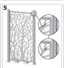
For each frame, drill four 1/8" holes through frame and into screen at provided locations. Fasten Decorative Screen to both frames using eight 3/4" screws (provided).
