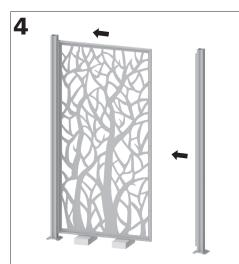
Insert Decorative Screen into frame on first post and use wood blocks to level Decorative Screen at desired height. Then move second post and frame into position to engage with other side of Decorative Screen.
