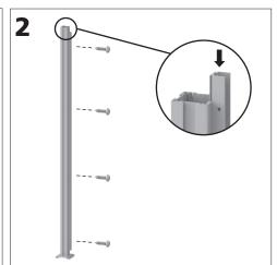
Slide first frame into slot on post and position at desired height. Ensure bottom of frame is at least 1" above top of post base. Drill four 1/8" holes through frame and into post at provided locations. Fasten frame to post with four 3/4" screws (provided).
